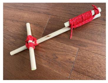
Cut three pieces of dowel rod, one 18", one 10" and one 6". On the 18" piece, carve a concave notch in the dowel rod 5" from one end to receive a 'cross' piece. On the 10" piece, drill and tap a hole in the middle or 5" from the end. In the 6" piece, drill and tap two holes 1 1/2" from each end. Also drill a hole in the middle of two pine hole plugs.
